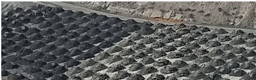
Figure 5 Filtered tailings on the drying platform
