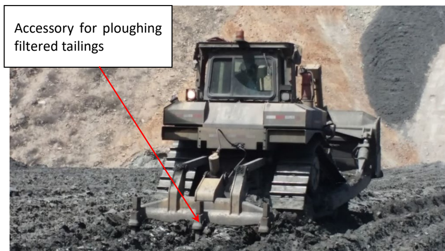
Figure 8 Ploughing process of filtered tailings
