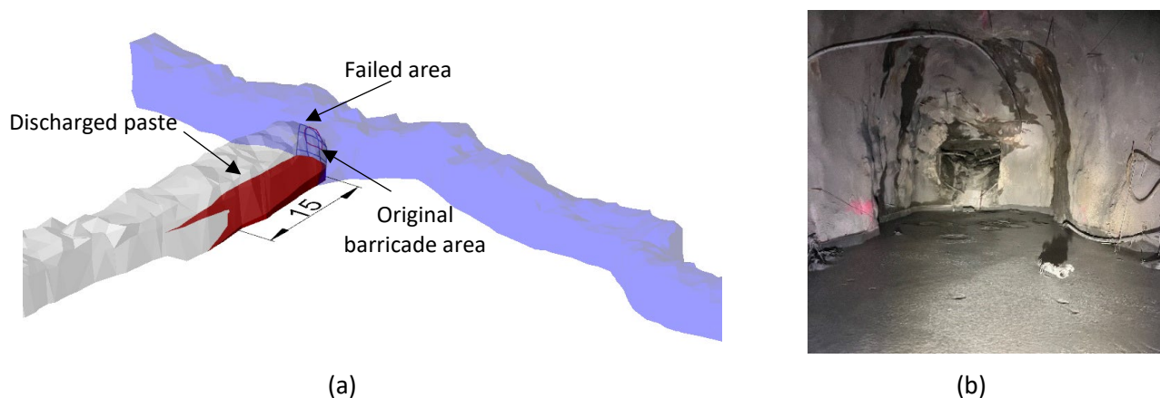
Figure 7 (a) Original barricade perimeter, failure area and paste discharged; (b) OLW_-330_-330_1_3 and -330_1_6 barricade failure and blocked Breather Pipe 5
