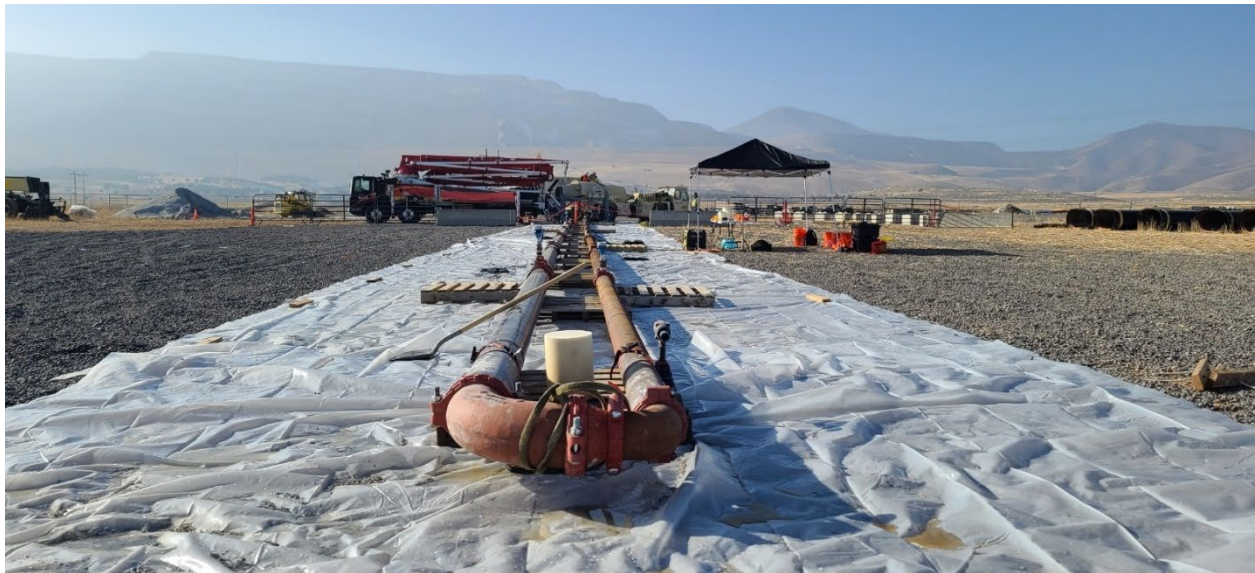
Figure 6 Flow loop testing installation
