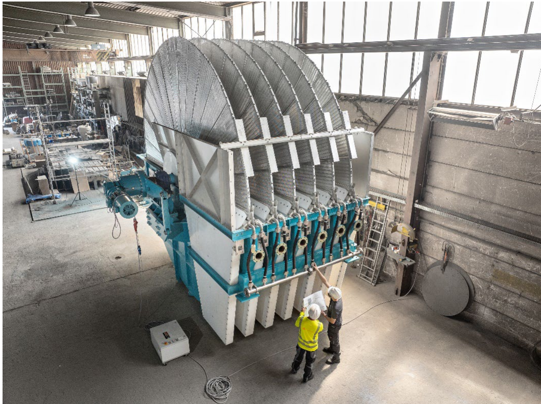
Figure 8 XL352 filter after the shop assembly and the dry test run
