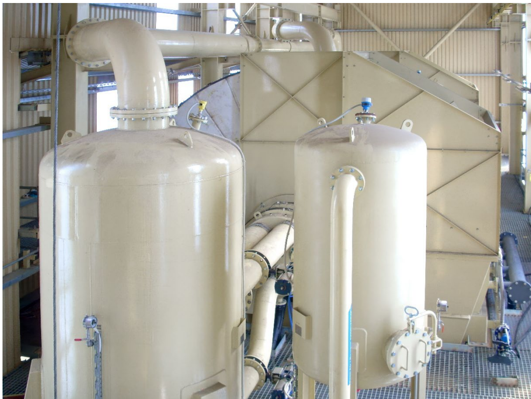
Figure 11 Two dewatering ports on a high-performance disc filter separating tailings
