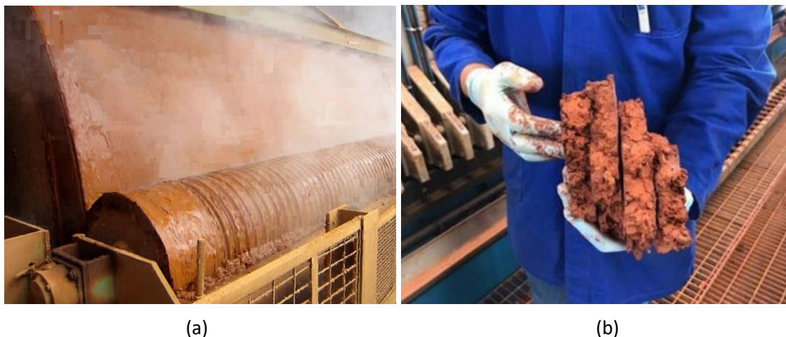
Figure 6 (a) Cake discharge vacuum drum filter; (b) Filter press cake ( p_{\text{abs}} = 6-7 \text{ bar} )
