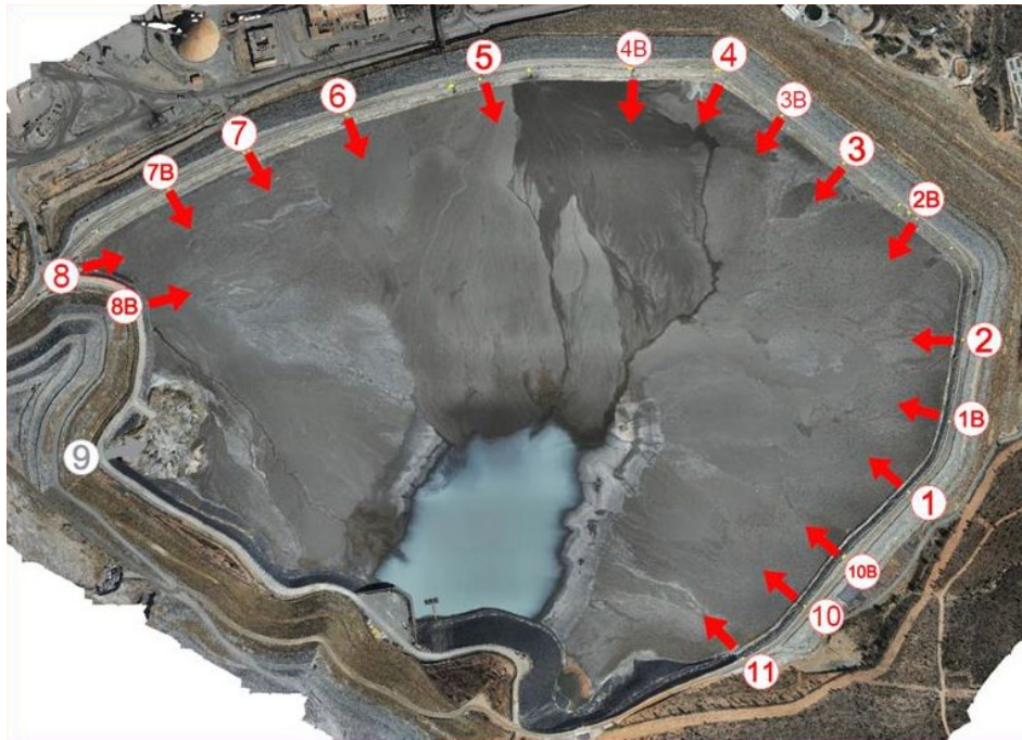
Figure 2 Spigoting installation for final landform
