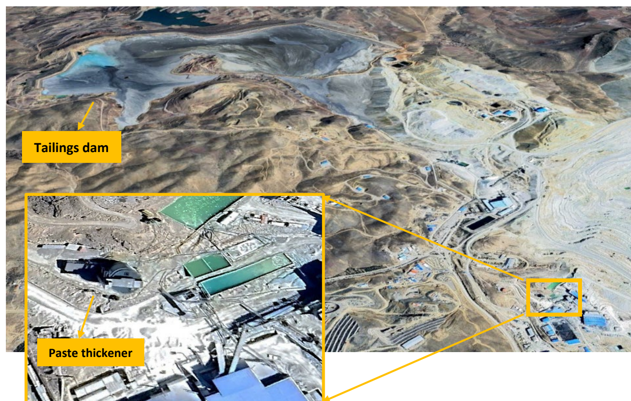
Figure 2 Tailings management in Rangin Felez copper mine
