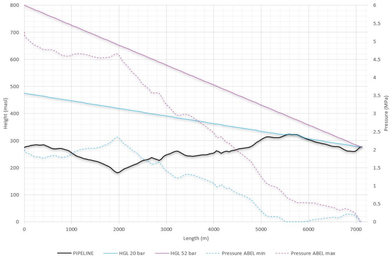
Figure 5 Hydraulic grade line (HGL) and pressure values in the new transport line
