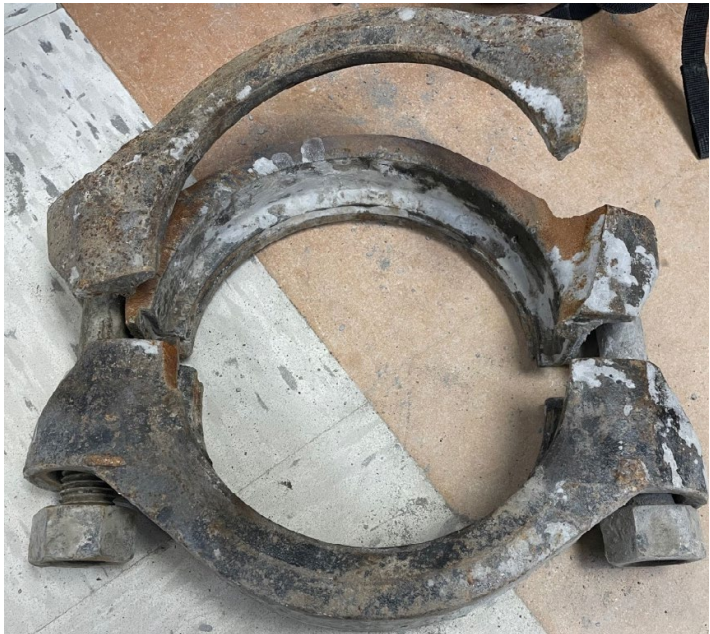
Figure 6 Mechanical end joint coupling failure (Correia & Jacobs 2024)
