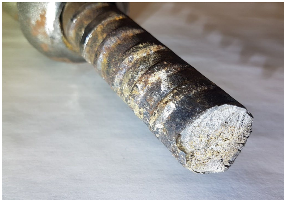
Figure 2 Rockbolt from underground distribution system support sheared by transient forces (McGuinness et al. 2021)
