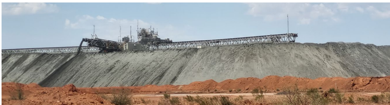
Figure 7 Filtered stack deposition
