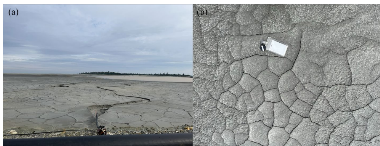
Figure 1 Desiccation cracks in (a) slurry and (b) filtered tailings
