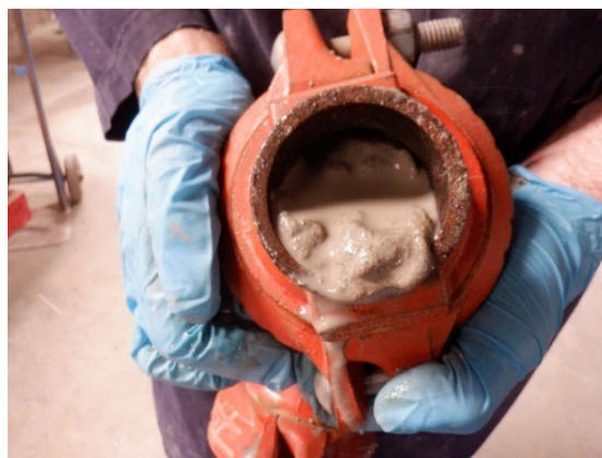
Figure 3 Water segregating from the paste
