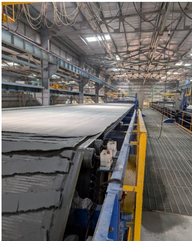
Figure 4 Horizontal vacuum belt filter discharge
