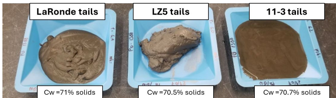
Figure 3 Comparative water-demand variation of the 3 mines at 70–71% solids (Noirant et al. 2023)
