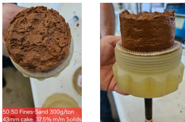
Figure 4 Effect of 300 g/tonne polymer addition on 50% fines, 50% coarse mixture subjected to vacuum filtration
