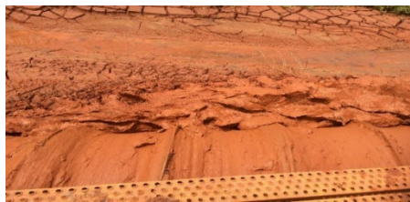
Figure 14 Paste build-up on the amphibious machine scrolls
