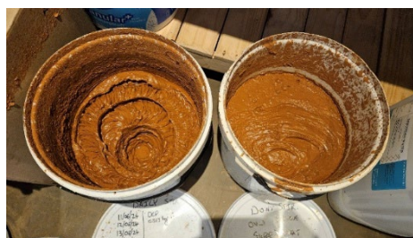
Figure 9 Buckets used to perform mechanical consolidation utilising varied mechanical stirring frequencies
