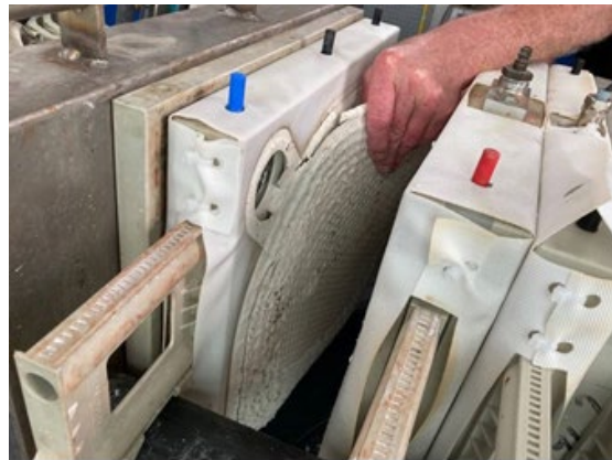
Figure 7 Filter press (size 470 × 470 mm) with 2 chambers including an AURUM membrane plate and a LENSER i-Plate with moisture sensor
