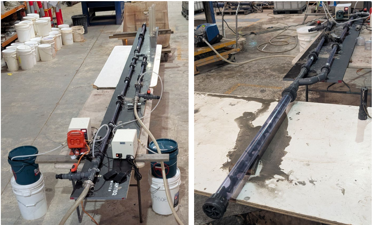
Figure 5 Static mixer rig set up
