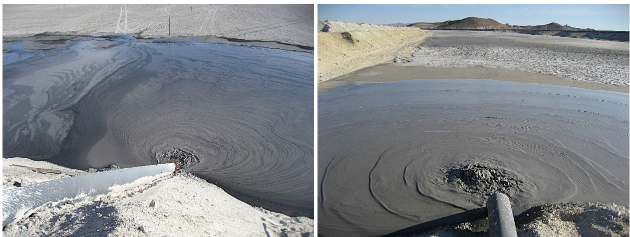
Figure 3 Stage 1 of beach formation. Sheet flow mechanism depositing a bed of fresh tailings
