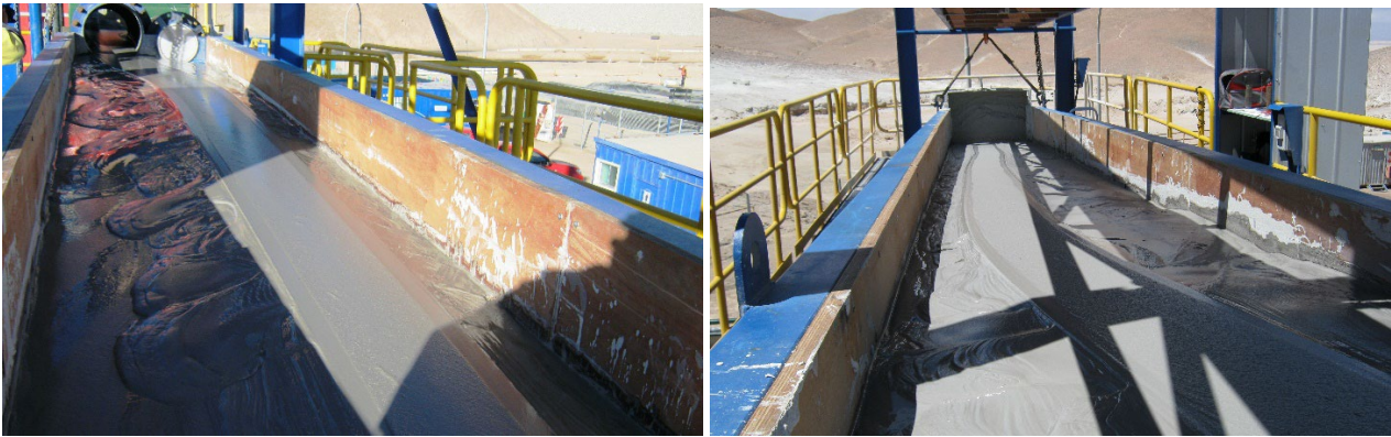
Figure 2 Channelisation of tailings during beach formation in a large-scale continuous flow flume trial, Copper mine
