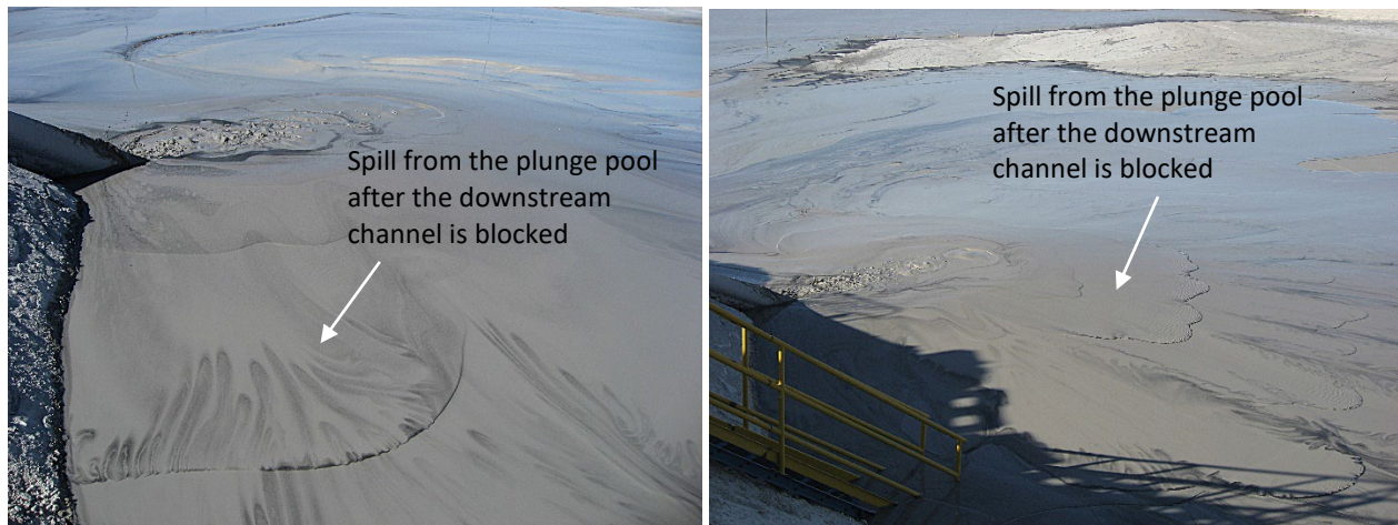
Figure 8 Stage 6 of beach formation. Sheet flow spills from the plunge pool to form a new channel toward a new direction
