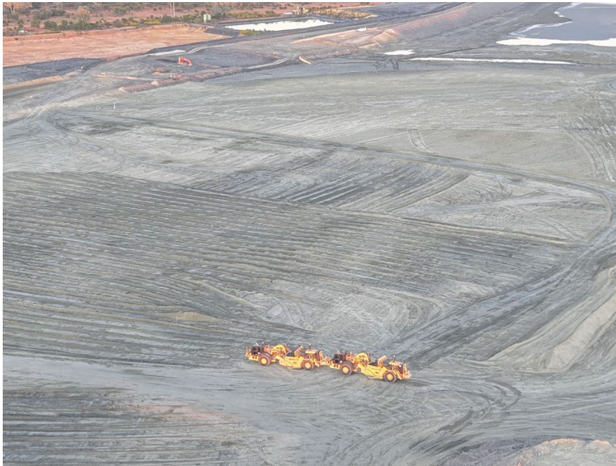
Figure 3 Open bowl scrapers on the east mound of the facility for tailings excavation
