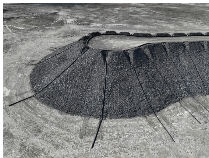
Figure 2 Tailings deposition spigots at the east causeway
