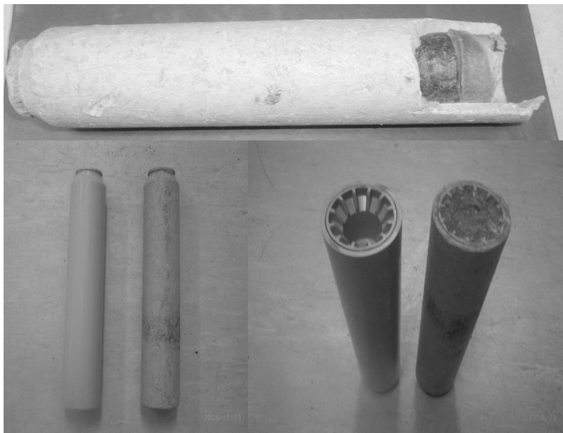
Figure 5 Photos show slightly damaged marker on top, uninstalled marker on the left, recovered marker on the right
