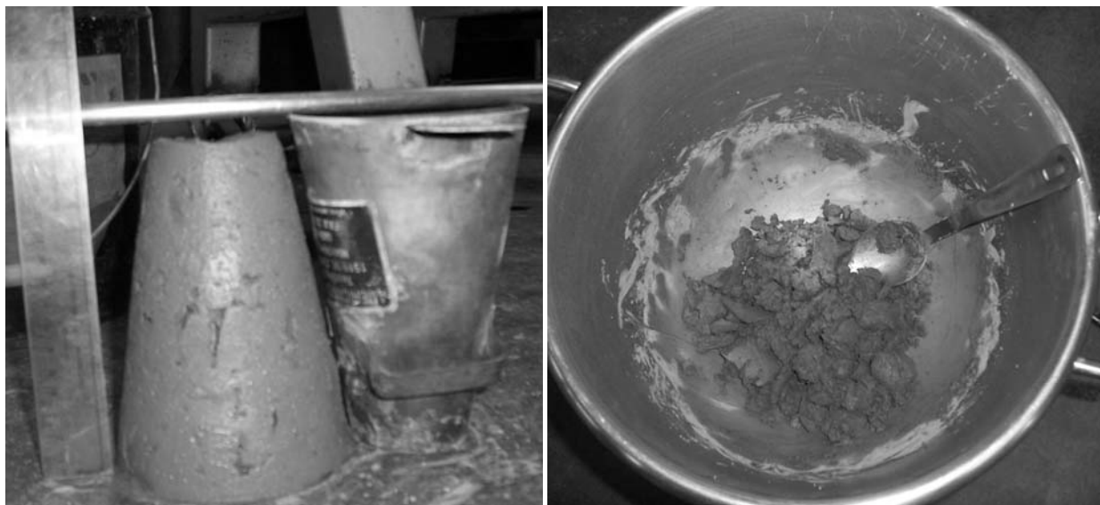
Figure 1 Pictures of cemented paste at 78%wt, mini-slump test (left) and tails aspect (right)
