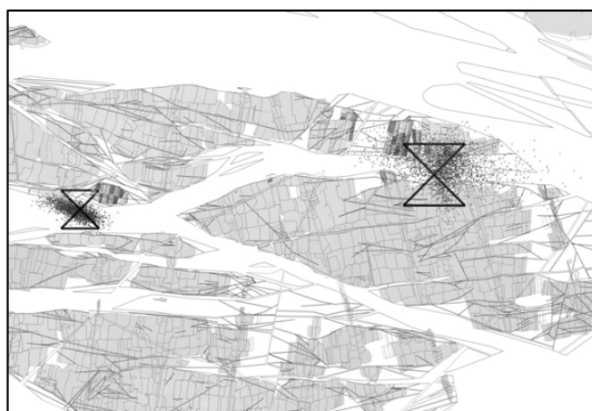
Figure 2 Seismic event locations from a view accounting for Z error. The crosses are the best locations, while the dots represent possible locations by varying P- and S-arrivals as well as velocities
