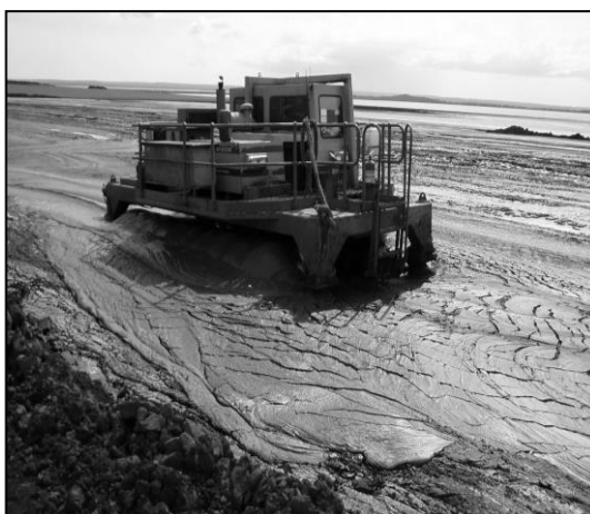
Figure 4 Amphirole (preparing a new mud farming area)
