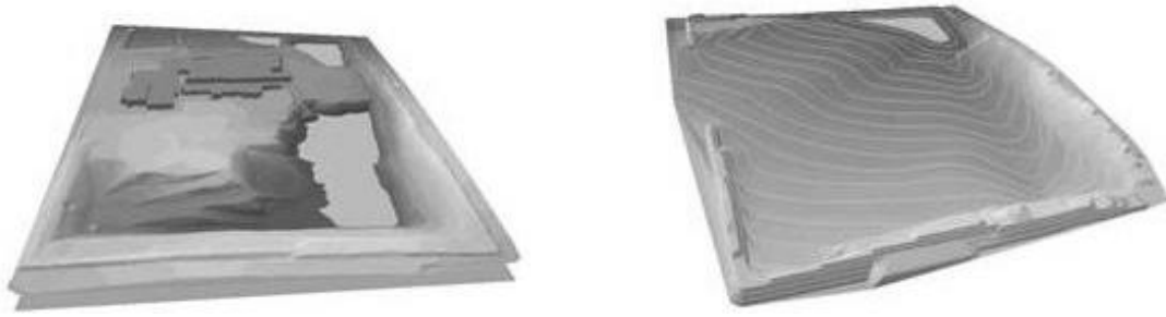
Figure 3 Left: Austral Bricks Scoresby existing site topography; Right: Austral Bricks Scoresby topography post filling operations
