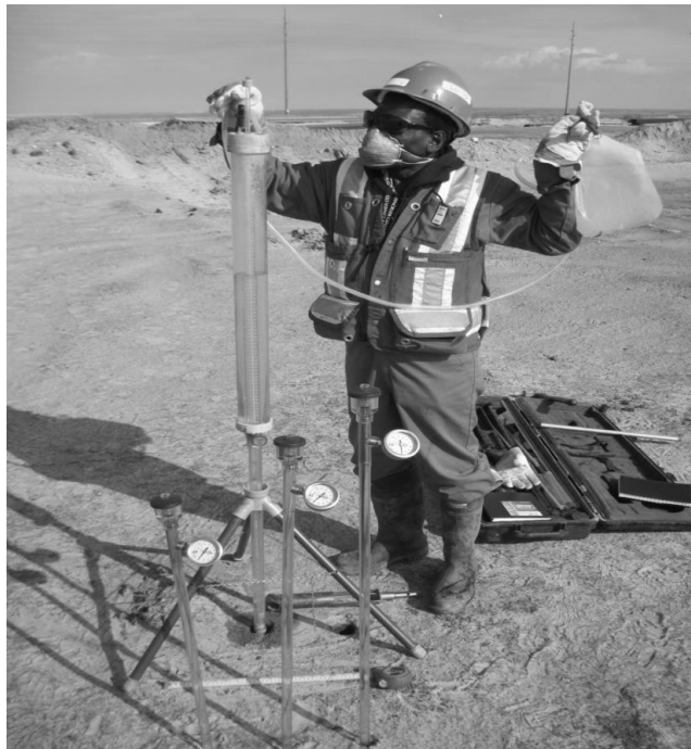
Figure 4 Measurements of hydraulic conductivity on the 2009 ILF-FFT deposit in Cell 3 at Syncrude's Mildred Lake Settling Basin using a Gulph permeameter
