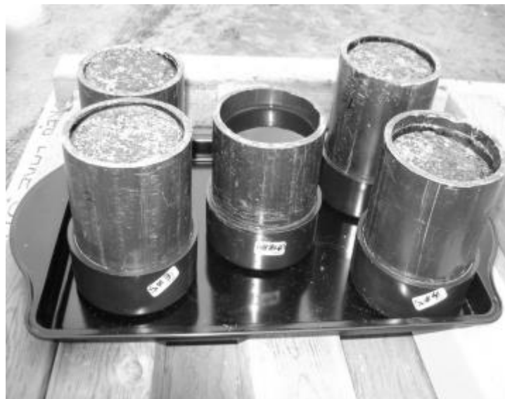
Figure 3 A set of 4" diameter PVC lysimeters used for evaporation measurements
