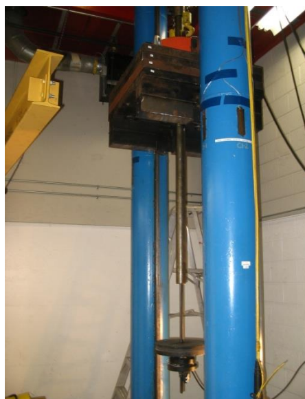
Figure 5 Drop test equipment and configuration at CANMET, Ottawa
