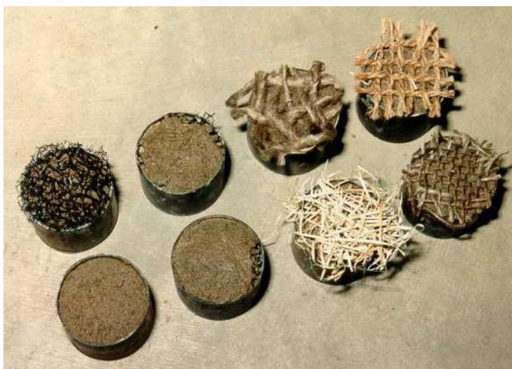
Figure 1 Ellison splash cups with geotextile treatments prior to rainsplash erosion tests using simulated rainfall. Top row (left to right: Enkamat (surface); Enkamat (buried); Geojute; Bachbettgewebe. Bottom row: Control (bare soil; no geotextile); Tensarmat; Enviromat; Fine geojute)
