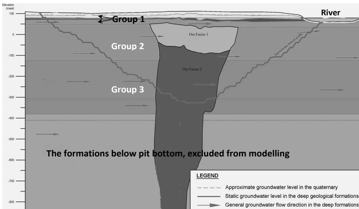
**Figure 5 Conceptual hydrogeological model cross-section of the diamond mine**
