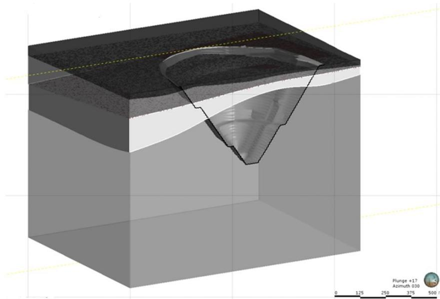
**Figure 2** Cross section west–east of the proposed pit shell. Zone in which inflows were detected depicted in white, the weathered zone in black and the remaining rock mass in grey
