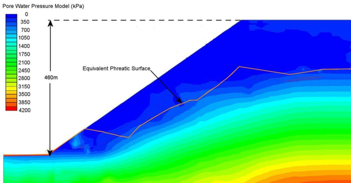
**Figure 7 Cross section of the pressure head achieved with the single 30 m spaced drains (vertical spacing of the four drain layers is 50 m)**
