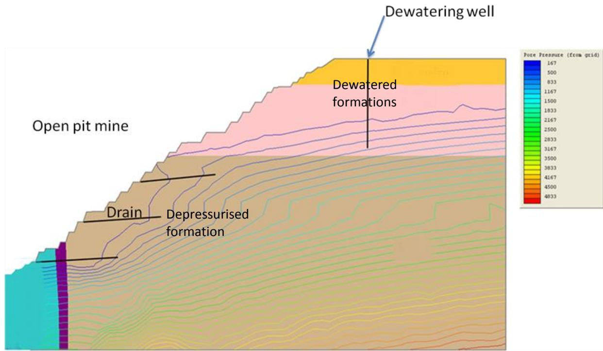
**Figure 1** Figure illustrating dewatering and depressurisation of pit wall formations
