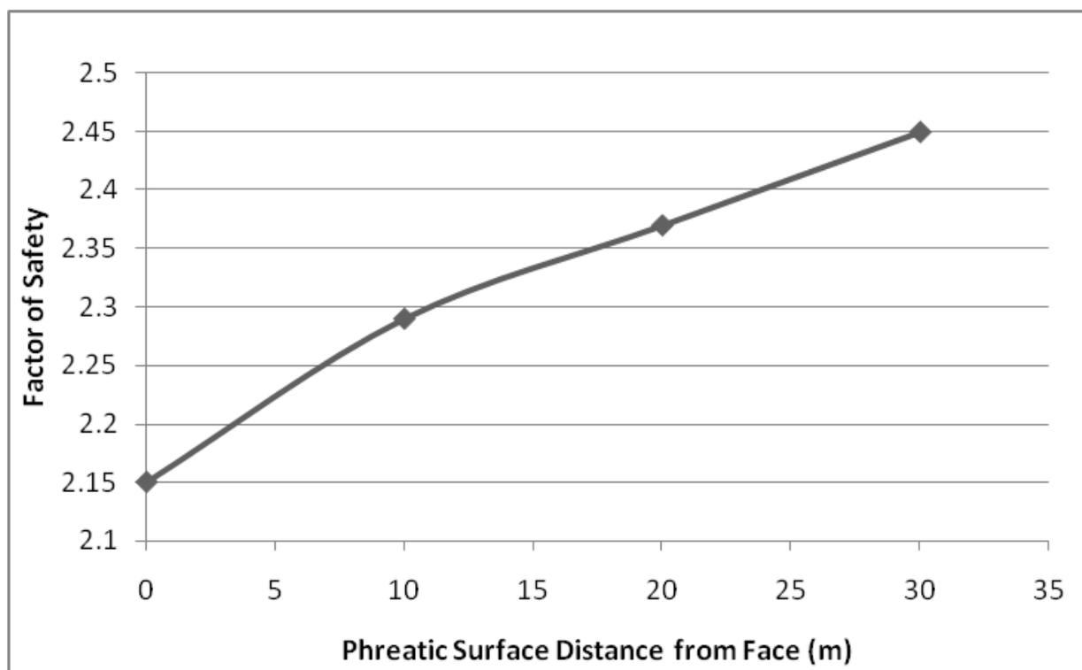
**Figure 4** Distance from face of phreatic surface versus Factor of Safety
