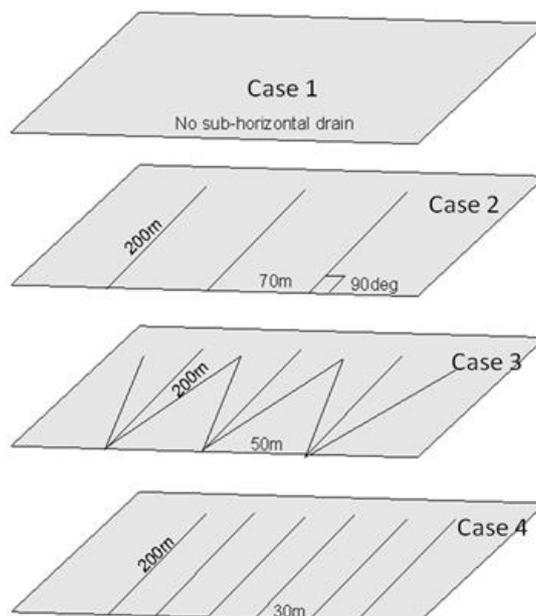
**Figure 6 Configuration of the sub-horizontal drains used to simulate depressurisation of Group 3 formation in the model**
