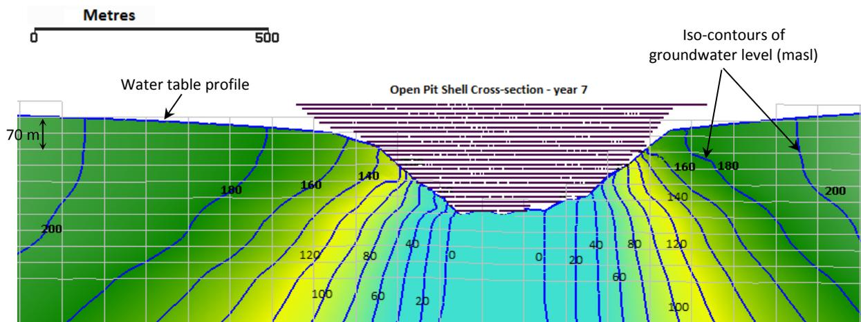
**Figure 3** Example of groundwater model results showing cross-section of pit shell and simulated phreatic surface
