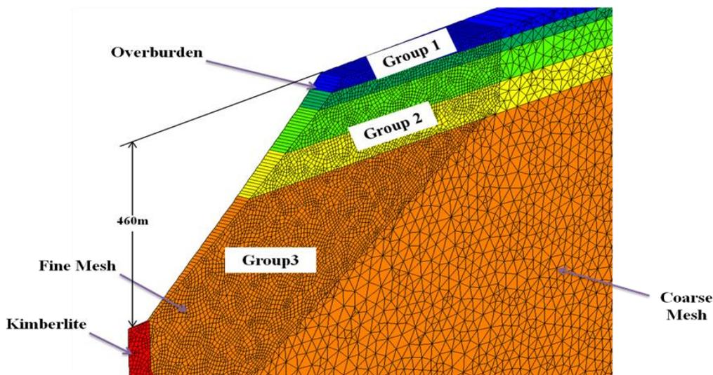
Figure 8 Geotechnical model setup – FLAC3D
