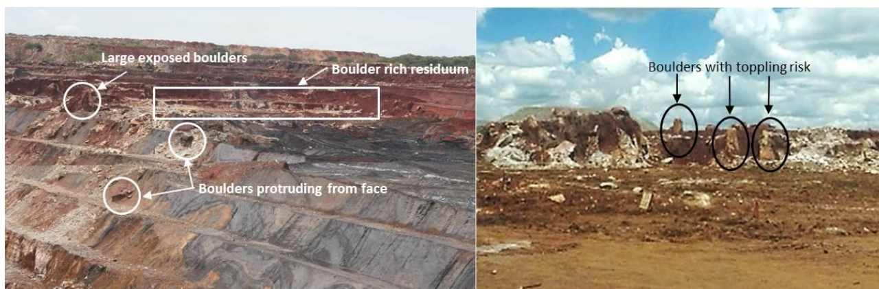
Figure 3 Protruding boulders in the northern cutback of North West Pit (left), boulders exposed on the mining area, at risk of toppling (right)
