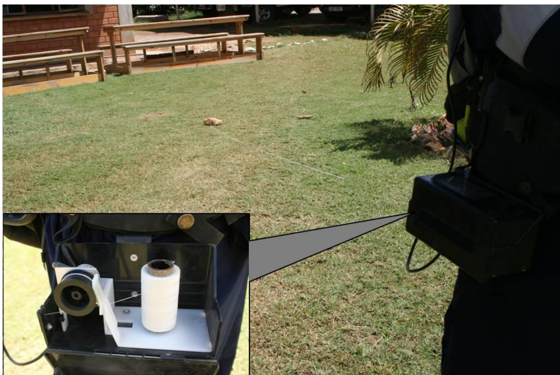
Figure 5 Hip-chain housing the thread, wound around the wheel to activate the recorder while walking each scan line
