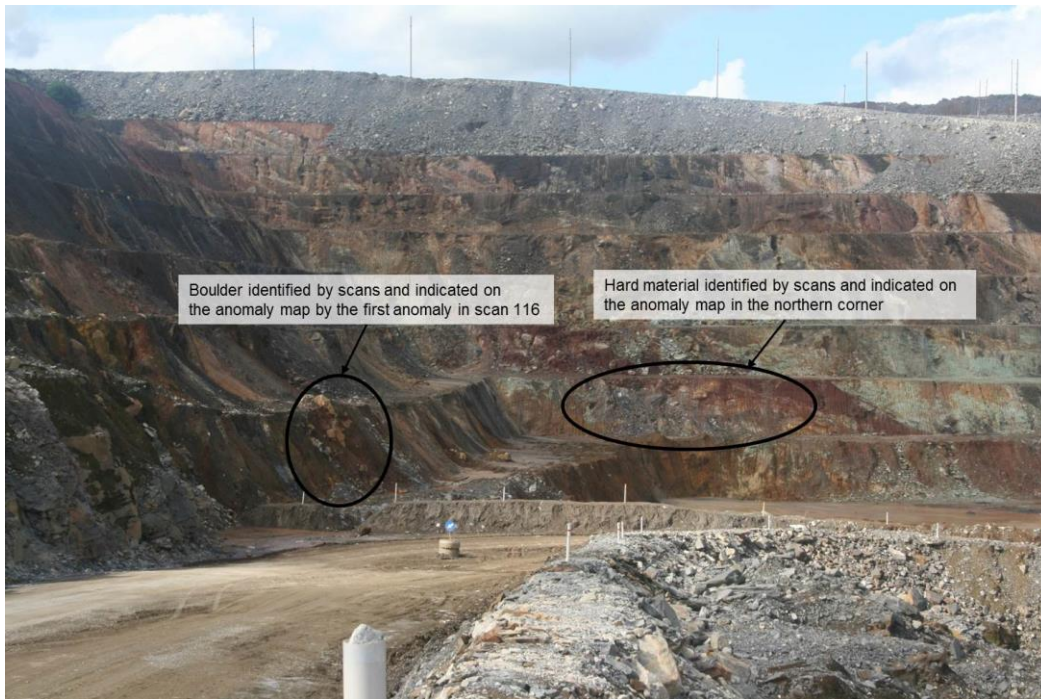
Figure 10 Image of the scanned area on completion of mining. Hard areas indicated by the radargrams are now visible on the benches
