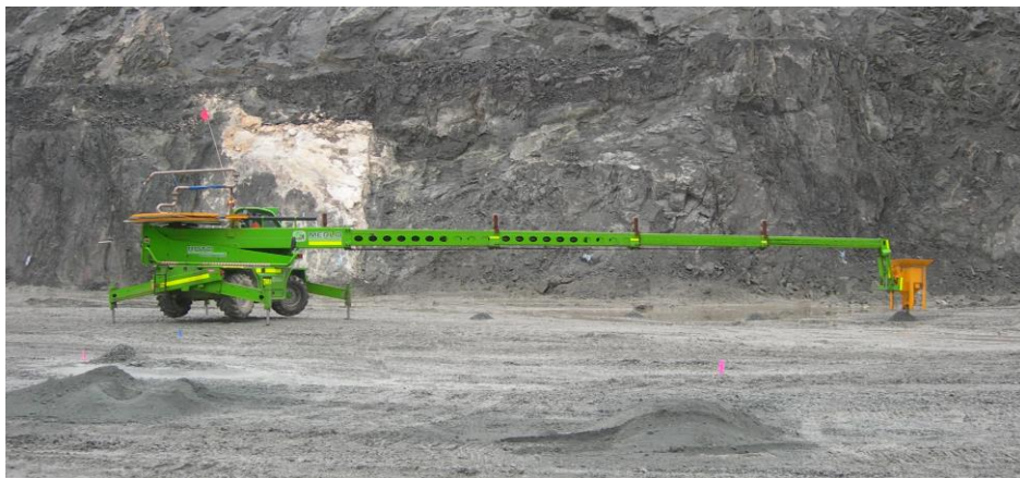
Figure 10 Grange Resource's patented Remote Explosive Blasting Unit
