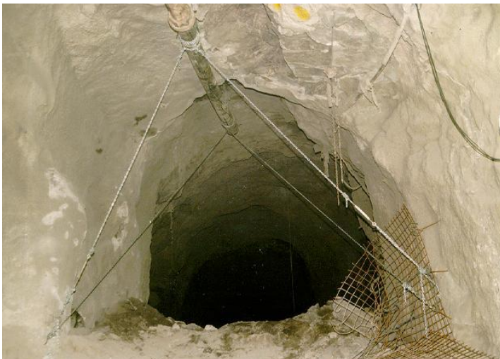
Figure 11 Stopes filled through horizontal pipes (left) and boreholes (right)
