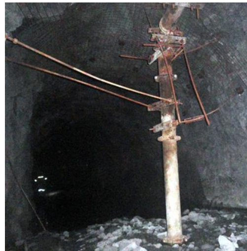
Figure 11 Stopes filled through horizontal pipes (left) and boreholes (right)
