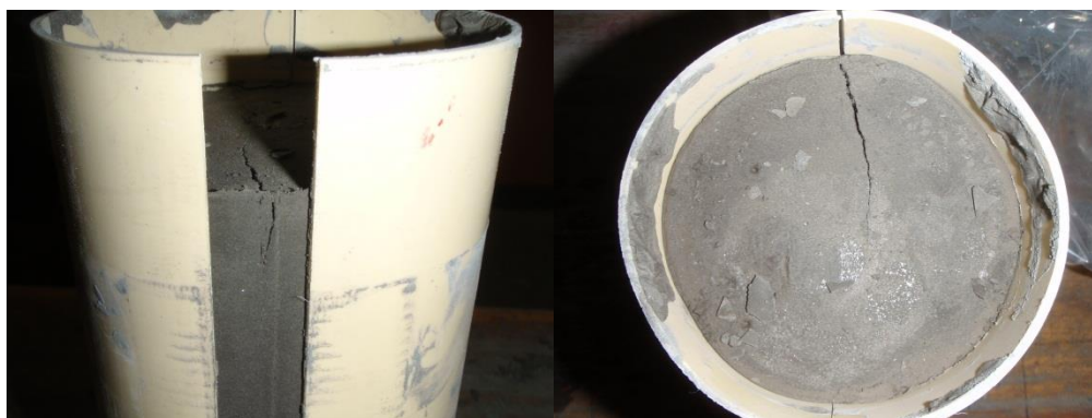
Figure 7 Shrinkage crack development on one gold tailings test set influencing the final results
