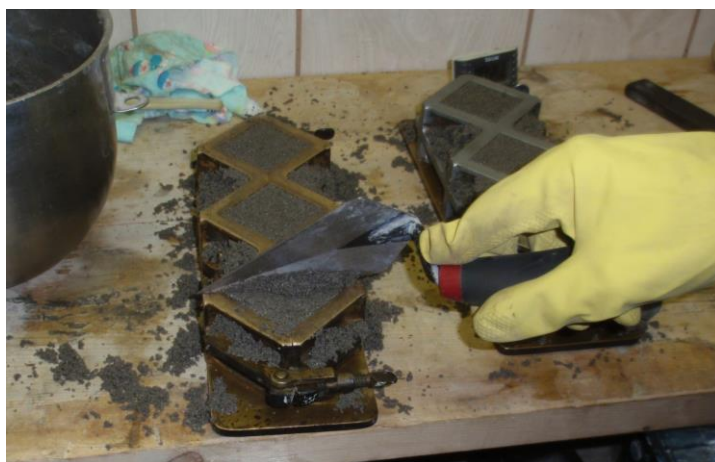
Figure 1 Samples were prepared in a temperature-controlled (5°C) room
