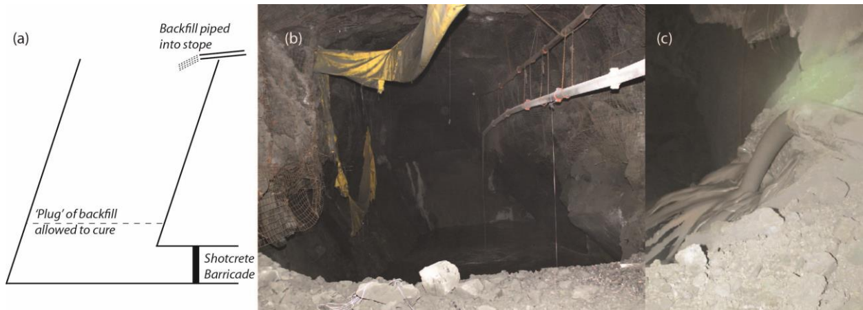
Figure 1 (a) schematic diagram of backfilling and backfilling with cemented; (b) hydraulic; and (c) paste fill
