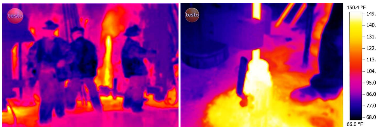
Figure 3 Thermal imaging of miners drilling grouting holes on the 1,969 m bench
