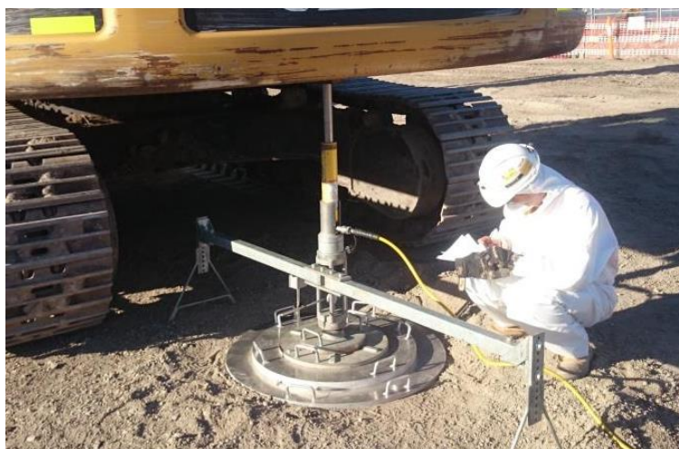
Figure 2 Simplified plate load test set up using a 1 m diameter plate
