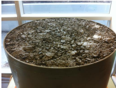
Figure 1 Large-scale oedometer test set up. Sample diameter is 300 mm
