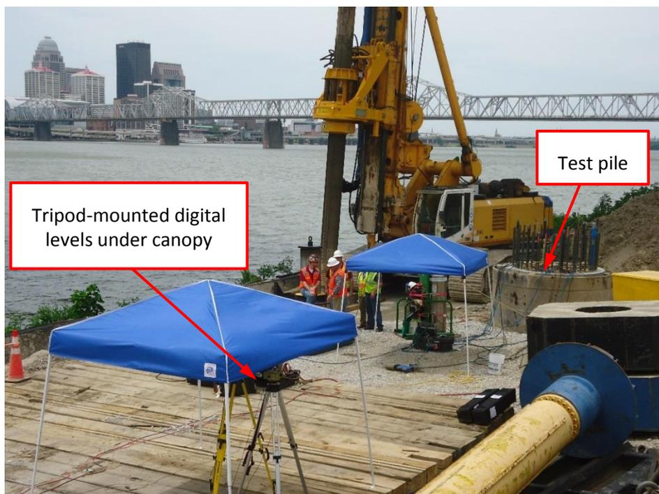
**Figure 9 Direct top of pile monitoring during O-cell test**
