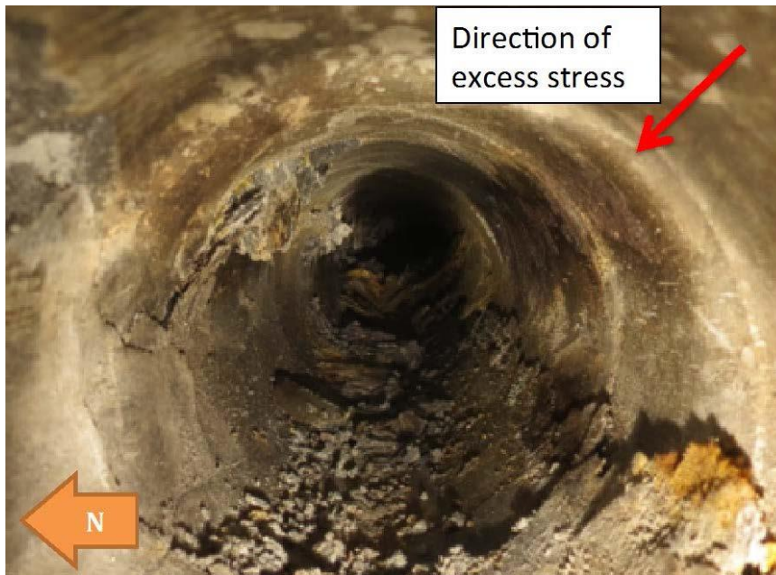
Figure 8 Borehole breakout (hole facing directly east along C Zone orebody strike)
