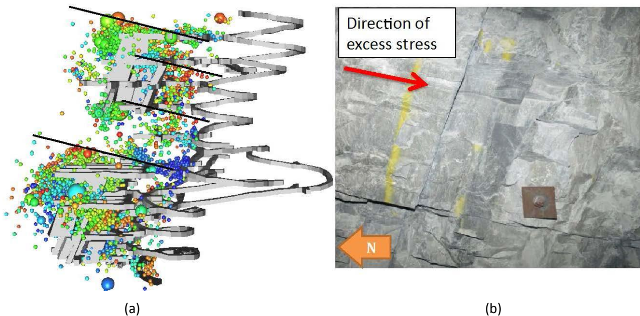
Figure 9 (a) formation of fractures as seen from seismic system; and (b) close up of stress induced fracturing. Both are viewed towards the east
