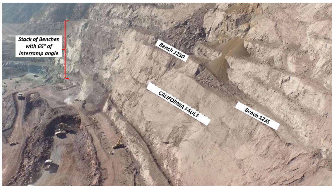
Figure 19 Development of 65° inter-ramp angle in the north sector of Phase 3 and Discharge California Fault plane between 1250 to 1175
