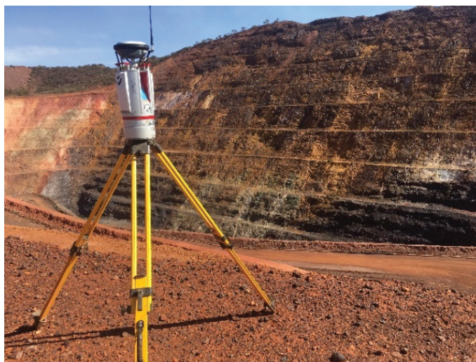
Figure 2 RIEGL laser scanner for surveying an opencast mine (RIEGL 2019a)
