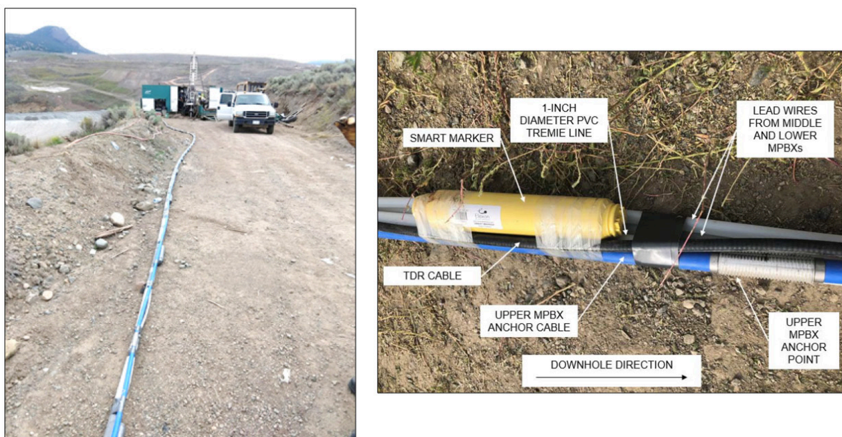
Figure 5 Preparation of the instrumentation string on surface (left) and description of the components (right)
