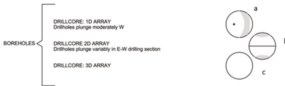
Figure 13 Blind zones for conventional borehole and mapping (after Laing 2005 in Fowler 2013)
