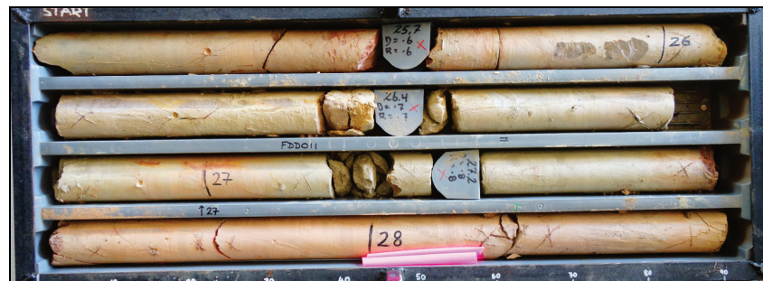
Figure 2 Highly weathered core with preserved rock texture
