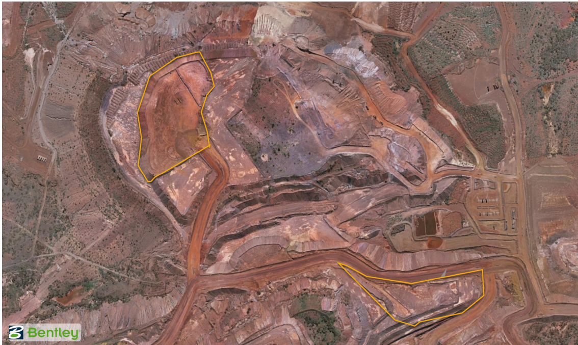
Figure 4 Encapsulation stockpile area located on the NEBC waste dump and additional waste material stockpile
