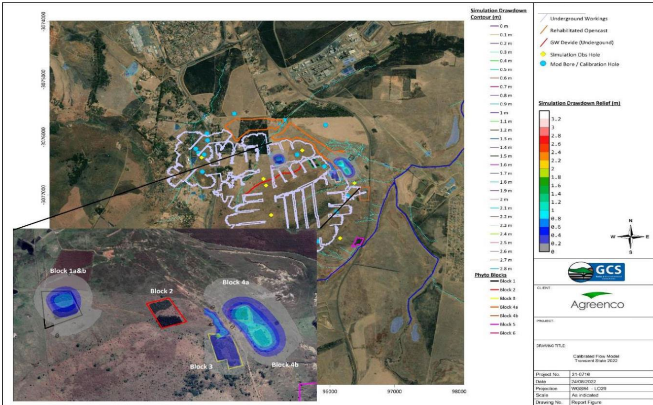
Figure 8 Transient state Re & ET model visual output (drawdown in the test block areas)
