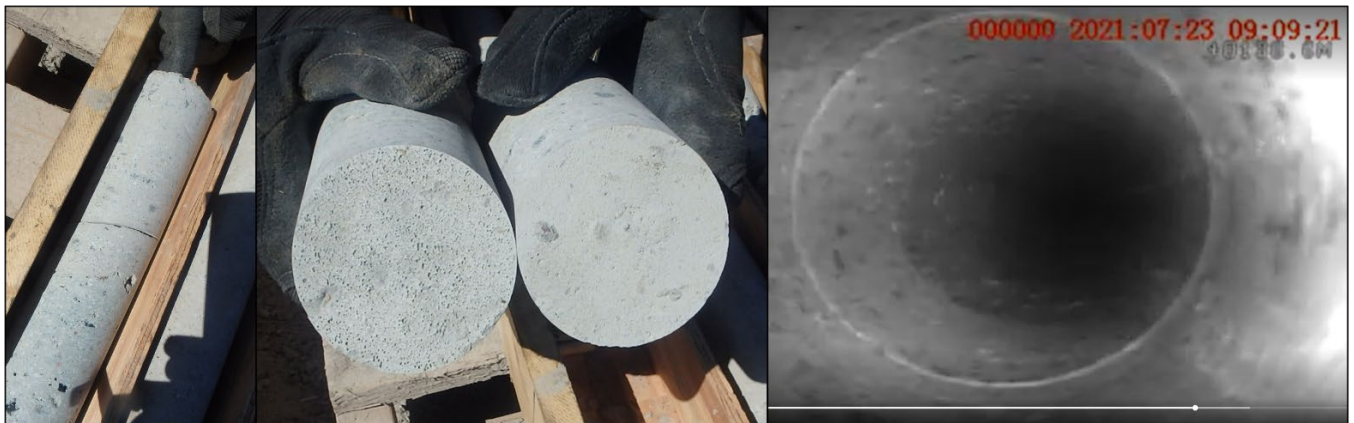
Figure 7 Interpreted cold joint in box (left), split to expose surfaces (centre) and in borehole camera video (right) from borehole 1 at ~138.7 m along hole/30.24 mamsl
