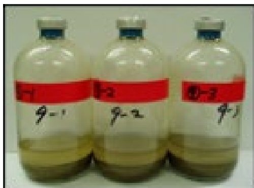
Figure 1 Photo of batch incubations with aquifer material and overlying groundwater; note that the incubations are not slurried (i.e. lower volume of water than solids)
