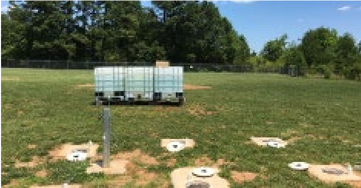
Figure 2 Field injection totes emplaced around well array for in situ microbial Fe(III), Mn(IV), and Cr(VI) reduction; field totes contained soluble electron donors (low molecular mass organic acids) derived from fermentation of higher molecular mass electron donors
