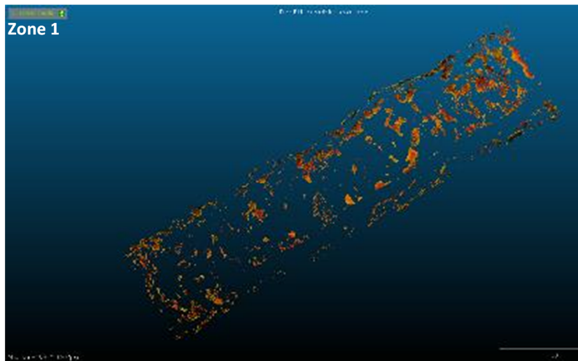
Figure 5 Comparison of the shape measured by LiDAR before and after a induced seismic event
