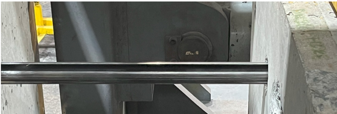
Figure 11 Condition of friction unit after axial loading and rupture of the bar
