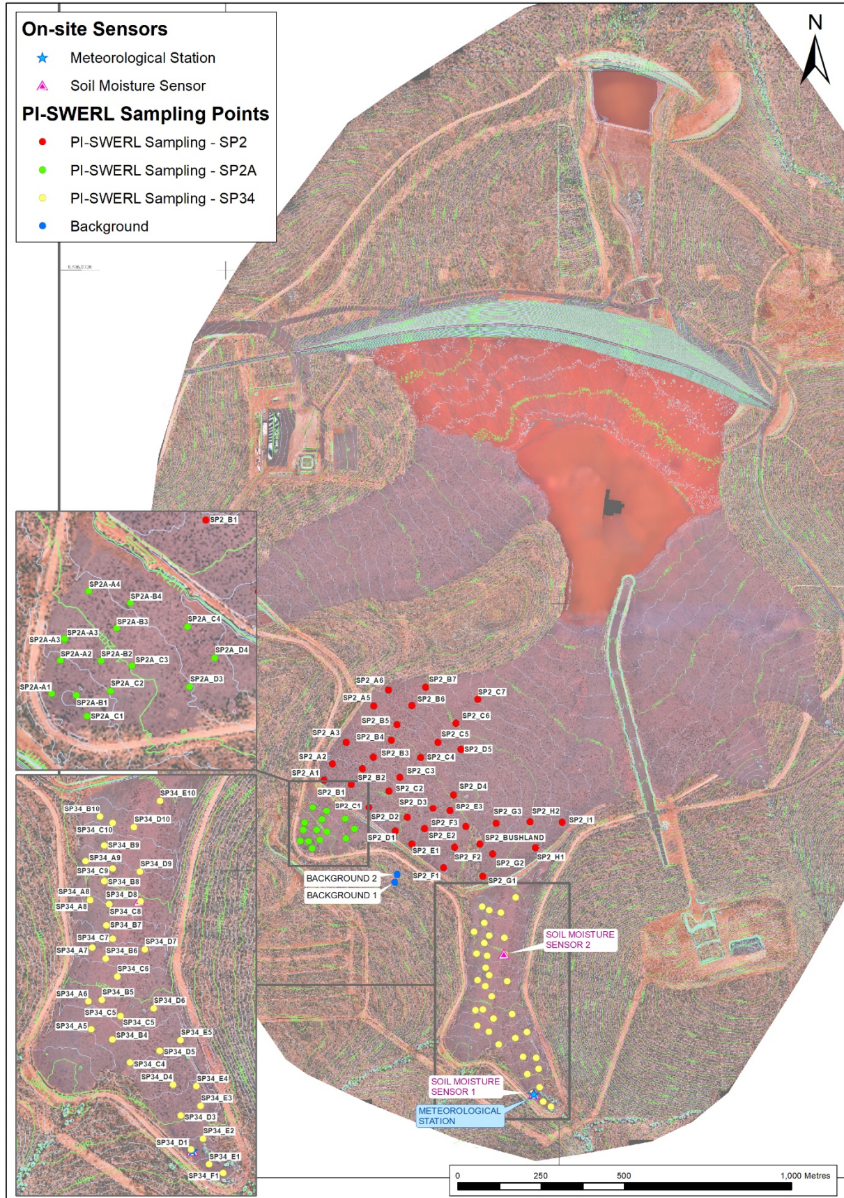
Figure 1 Tailings storage facility sampling locations at sampling point (SP) 2A (green), SP2 (red) and SP34 (yellow)
