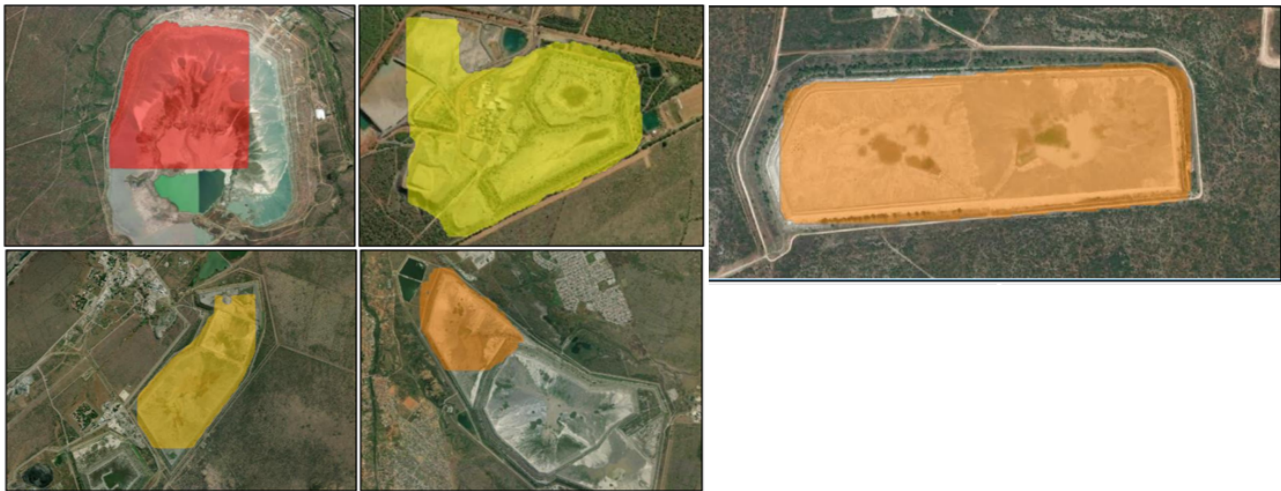
Figure 8 Sample results of the tailings storage facility object detection by Mask RCNN
